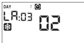
6. Once all parameters are set, to exit and go back to the programming menu, press for a short time the key **SET**.
