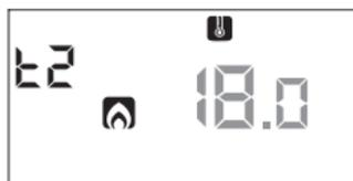
5. The value of the flashing T3 temperature is displayed. Modify the value with the keys ▲ and ▼ and press the key ⏴ to go back to the page of T1 temperature.
