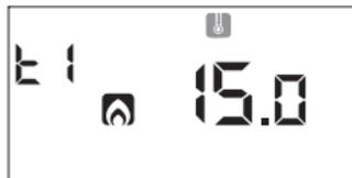
3. The value of the flashing T1 temperature is displayed. Modify the value with the keys ▲ and ▼ and press the key ⏴ to move to the modification of T2.
