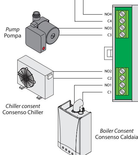
Connect the controller by using wires far from main power line (24 Vac / 230 Vac) to avoid interference.
