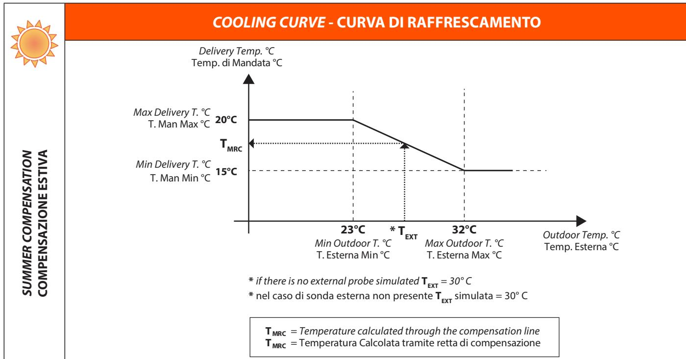
During the calculation stage, in summer mode, the controller will calculate the temperature  $T_{MRC}$ , i.e. the temperature calculated through the compensation line, considering the outdoor temperature  $T_{EXT}$  detected.
