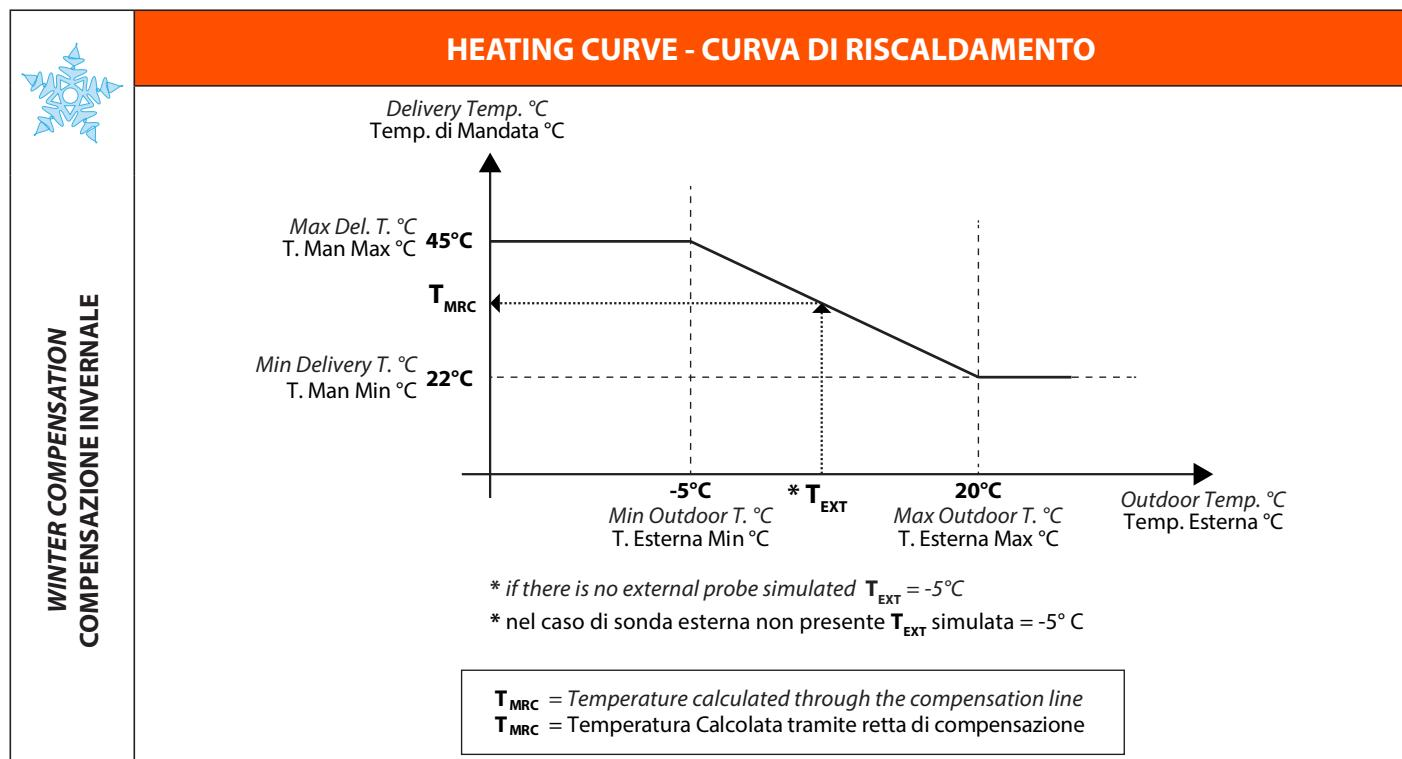
During the calculation stage, in winter mode, the controller will work out a temperature **T<sub>MRC</sub>**, i.e. a temperature calculated through the compensation line, considering the outdoor temperature **T<sub>EXT</sub>** detected.
