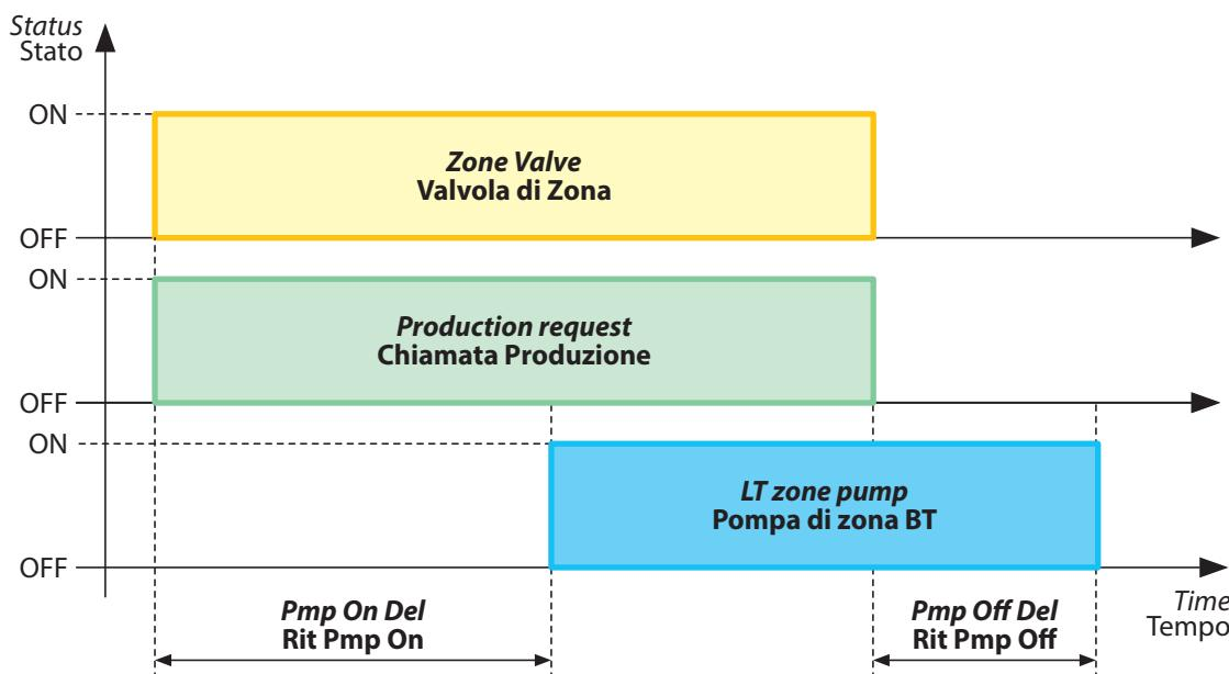
Therefore, the **Production Request** input starts together with the zone input or with the dehumidification input.
