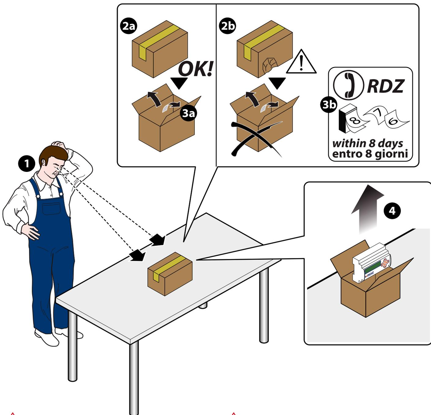
The remote control packaging must be removed with care, ensuring that the control unit is not damaged. The materials which make up the packaging are different: wood, cardboard, nylon etc. Store them separately and deliver them for disposal or, where appropriate, recycling, to the relevant companies, thus reducing the environmental impact.
