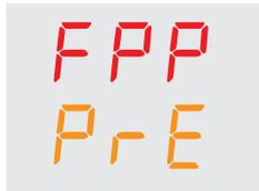
Through the controller on the machine Set the parameter "Free-Cooling Selector" to: PRE
