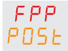
Through the controller on the machine Set the parameter "Free-Cooling Selector" to: POST
