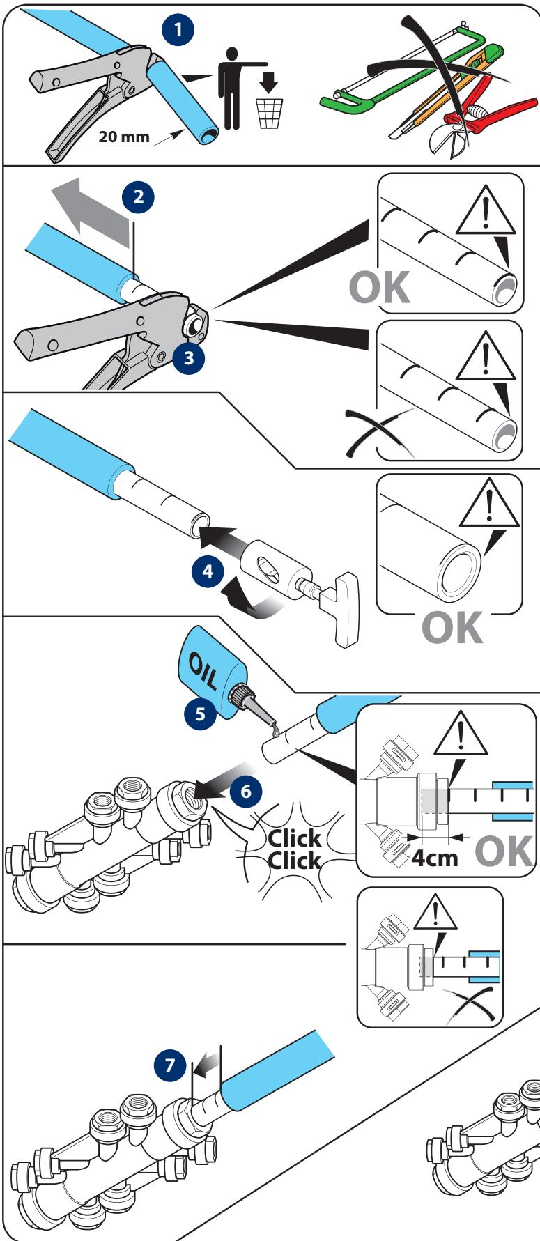
Cut the exceeding sheath by using a pipe cutter
