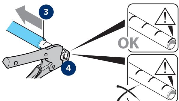
Make the sheath run over the pipe and move it away from the cut.
