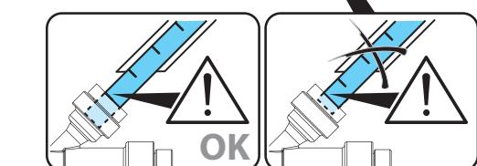
Introduce the pipe, making sure that the next mark coincides with the fitting edge.
