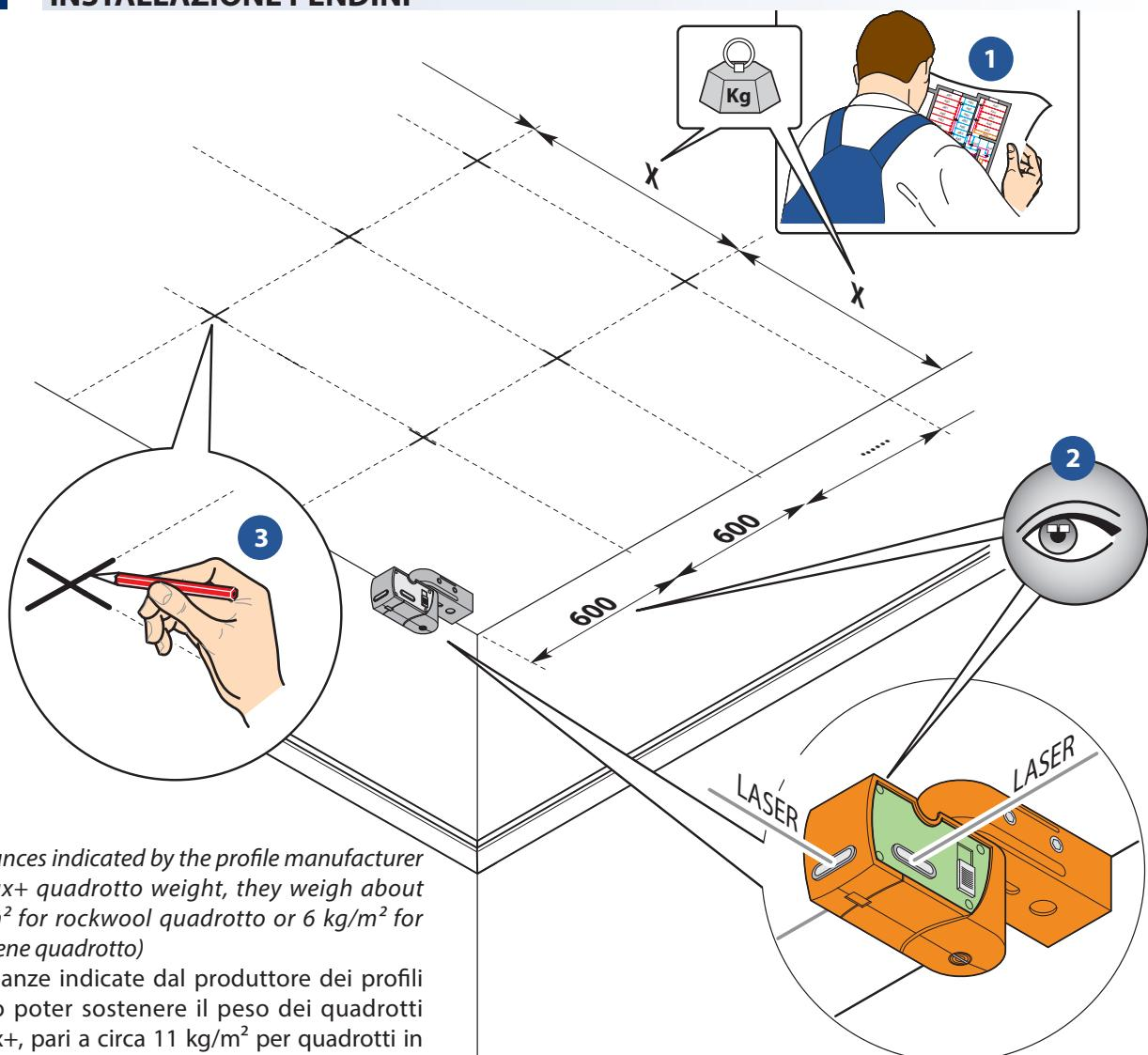
**X** = distances indicated by the profile manufacturer (b!klimax+ quadrotto weight, they weigh about 11 kg/m<sup>2</sup> for rockwool quadrotto or 6 kg/m<sup>2</sup> for polystyrene quadrotto)
