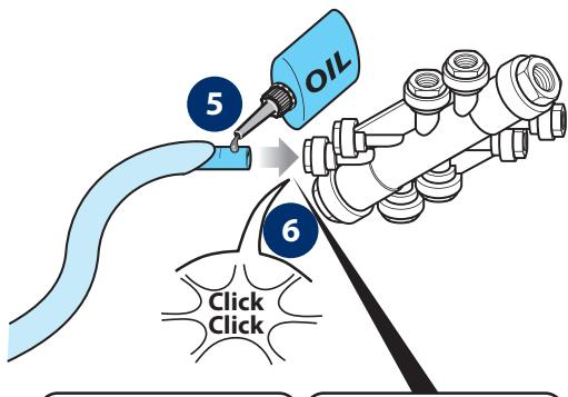
Cut the pipe on the tally mark; in this way you can easily check the right installation of the pipe (see stages 6).
