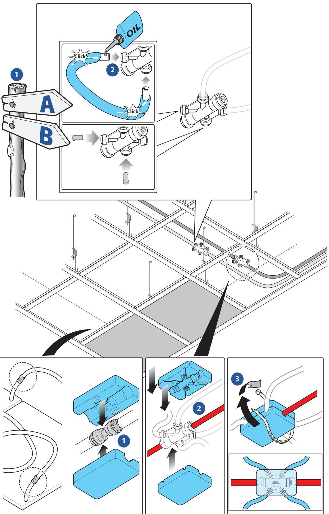
**14****INSTALLATION OF INSULATING SHELLS
