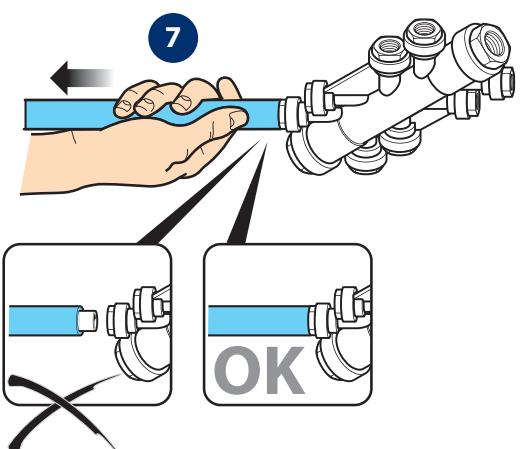
Check the right installation of the pipe into the fitting by pressing it out softly.
