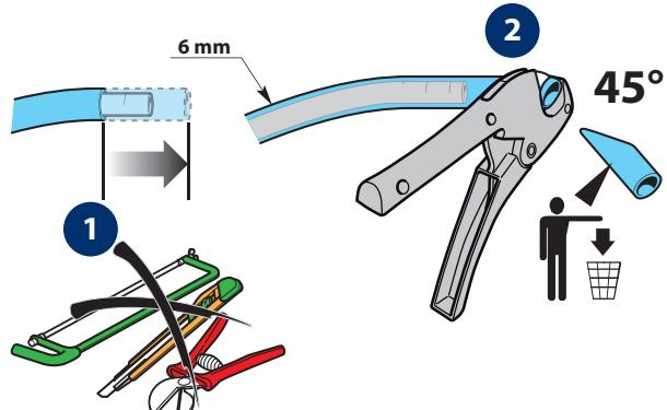
Cut the exceeding sheath by using a pipe cutter; the cut should be done with 45° inclination.
