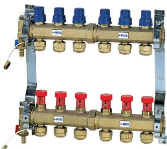
*CONTROL manifolds Ø 1 ¼" are made of brass, and they are used to distribute pipes into the rooms. They are provided with shut-off valves (suitable for electrothermic heads), micrometric lockshield valve with data labels to locate rooms, ball air vent valves and ball waste valves with hose nozzles and plugs, brackets with vibration damping rubber tops, which can be installed into cabinets or onto the wall, and fittings for polyethylene pipes Ø 20-16.*
