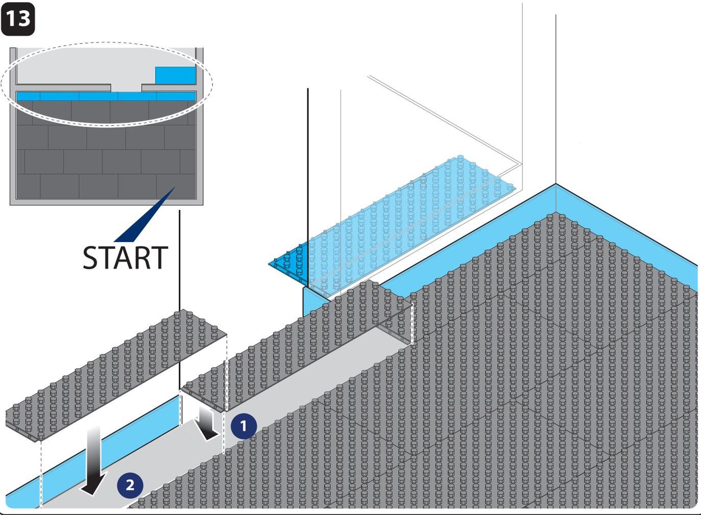
3.5 INSTALLATION OF THE PIPE RDZ CLIMA PB - POSA TUBO RDZ CLIMA PB
