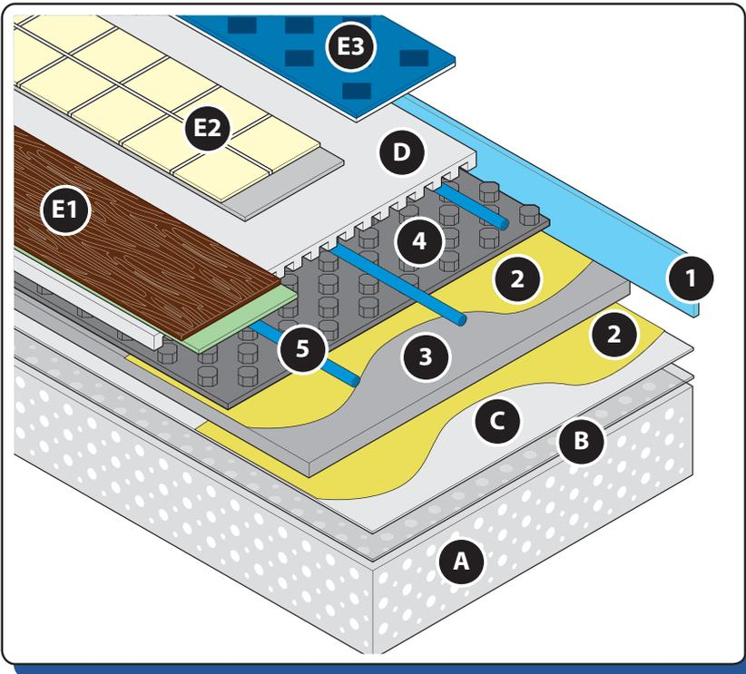
(\* The Extruded Panel must have a compression resistance  $\geq 400$  Kpa and must be glued both to the substrate and to the Super D panel.
