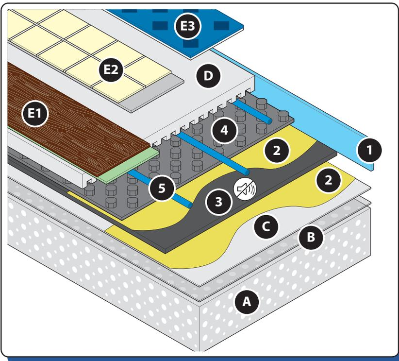
(\* The Acoustic Mat must be glued both to the substrate and to the Super D panel and the thickness of the special screed D must be increased ( $\geq 2$  cm).
