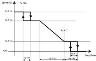
The fan speed can be controlled via analog/digital outputs or, alternatively, via serial on the same serial of the modulating compressor. Please see paragraph 11.5 for changing the parameters.
