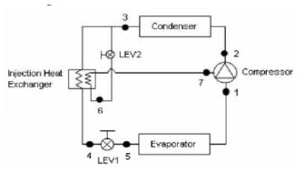
In the above drawing it is shown a simplified diagram of a refrigerant circuit that uses injection mono-compressor and intermediate exchanger with injection "economizer". The purpose of the injection is to obtain an "intermediate" cooling of the compressor in order to contain the discharge temperature below the critical values and allow it to operation even with very high compression ratios (for example, particularly with very low outdoor temperature and high temperature of the produced water).
