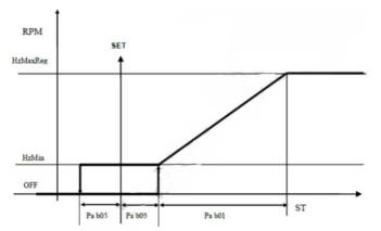
The following curve shows the adjustment without integral component (**b07** = 0)
