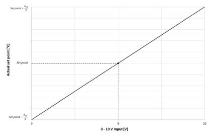
The 0-10V signal must be applied to the terminals AI10+ and AI10- (see the wiring diagrams).
