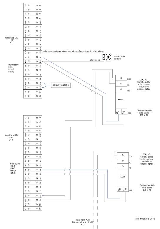
**NOTE:** turning off the unit remotely (onoff-onoff terminals), or by the on board keyboard, or by a remote keyboard does not affect the DHW operating mode. Once the **H10** parameter is set to be **1**, the unit switches to DHW priority as soon as powered. The on board display shows the temperature measured by the sensor placed inside the DHW water tank. Once the DHW cycle is completed, the display returns to show the outlet water sensor temperature.
