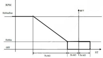
The following curve shows the adjustment without integral component (**b07** = 0)
