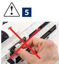
To remove the board insert a screwdriver in the hole to the left of Ethernet interface and pull up. **Do not remove the board by pulling the Ethernet connector.**
