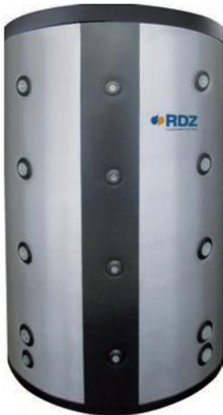
Buffer tank for heating water with stratification and instant DHW heat exchanger (removable) made of copper with 3-m<sup>2</sup> surface. Polyurethane foam insulation, thickness 100 mm. The heat exchanger makes it possible to produce domestic hot water instantly, and it does not need disinfection cycles. Ideal application with heat pump. Available in 2 versions:
